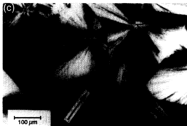
Figure 2 Growing of the crystal front of the \beta -modification ( T_c = 125^\circ\text{C} ) on vacuum bubbles formed in the encapsulated melt (a and b) and the residual structure after separate melting of the \beta -phase at 158^\circ\text{C} (c)
