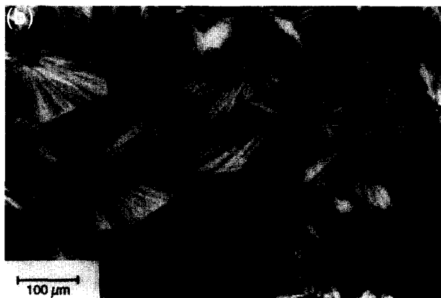
Figure 7 Twin spherulites formed during the \alpha - \beta transition on the surface of \alpha -spherulites growing in the encapsulated melt at T_c = 120^\circ\text{C} (a), and the residual structure after the separate melting of the \beta -phase at 158^\circ\text{C} (b)
