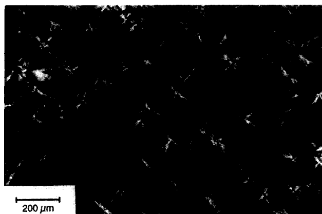
Figure 1 Formation of crack-like material-deficient boundaries between spherulites during high-temperature crystallization ( T_c = 135^\circ\text{C} )
