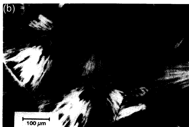
Figure 1 Formation of crack-like material-deficient boundaries between spherulites during high-temperature crystallization ( T_c = 135^\circ\text{C} )
